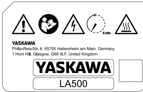
Figure 1.3 Warning Label “Risk of electric shock”
