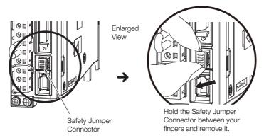
Connect the safety function device to the connector for the safety function device (CN8).
