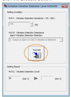
The newly set vibration detection level will be displayed and the value will be saved in the SERVO-PACK.
