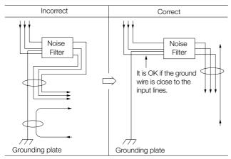
• Connect the Noise Filter ground wire directly to the grounding plate. Do not connect the Noise Filter ground wire to other ground wires.
