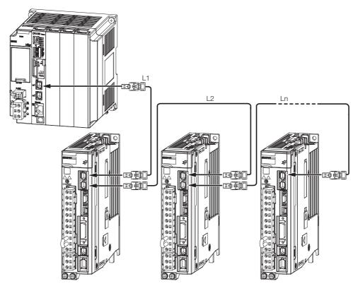
Note: The length of the cable between stations (L1, L2,  $\dots$  Ln) must be 50 m or less.
