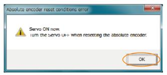
Click the **OK** Button. The Main Window will return. Turn OFF the servo and repeat the procedure from step 1.
