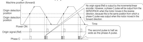
When Passing the First Origin Signal (Ref) in the Reverse Direction and Returning after Turning ON the Power Supply
