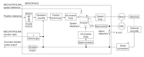
$<sup>\</sup>ensuremath{^{*}}$  The connected device depends on the type of external encoder.
