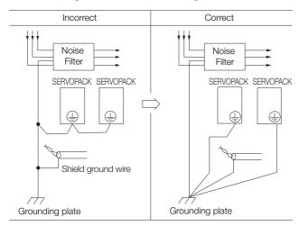
• If a Noise Filter is located inside a control panel, first connect the Noise Filter ground wire and the ground wires from other devices inside the control panel to the grounding plate for the control panel, then ground the plate.
