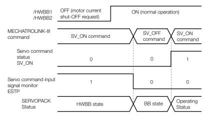
Note: If the SERVOPACK is placed in the BB state while the main circuit power supply is OFF, the HWBB state will be maintained until the SV\_OFF (Servo OFF: 32h) command is received.
