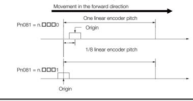
Observe the following precaution if you set Pn081 to n. \$\square\$ (Output phase-C pulses only in the forward direction).
