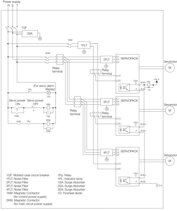
To comply with UL/cUL standards, you must install a branch circuit protective device at the power supply input section to each SERVOPACK. Refer to the following manual for details.  $\Sigma$ -7-Series  $\Sigma$ -7S/ $\Sigma$ -7W/ $\Sigma$ -7C SERVOPACK Safety Precautions (Manual No.:TOMP C710828 00)
