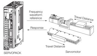
Easy FFT is built into the SERVOPACK for compatibility with previous products. Normally use autotuning without a host reference for tuning.
