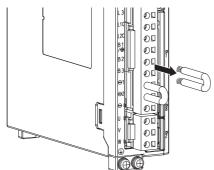
2. Connect the External Regenerative Resistor between the B1/⊕ and B2 terminals.
