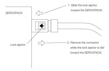
Note: The MECHATROLINK-III Communications Cable connector may be damaged if it is removed without being unlocked.
