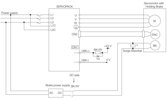
BK-RY: Brake control relay 1D: Flywheel diode
