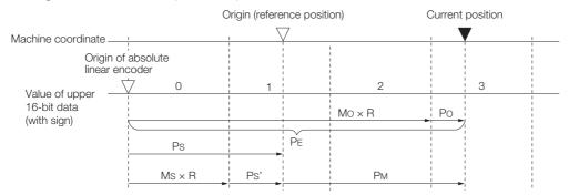
6.9.7 Alarm Output from the Output Ports for the Position Data from the Absolute Linear Encoder
