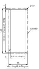
SGD7S-3R8A, -5R5A, -7R6A: 1.6 kg SGD7S-2R8F: 1.5 kg Unit: mm • Three-phase, 200 VAC: SGD7S-120A
