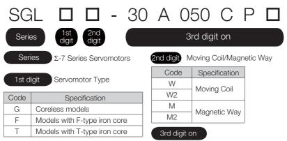
The specifications for the 3rd digit on depend on the Servomotor type.
