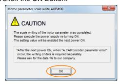
12. Turn the power supply to the SERVOPACK OFF and ON again.
