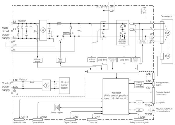
• Optional Specifications: Single-Phase, 200-VAC Power Supply Input (SERVOPACK Model: SGD7S-120A20A008)
