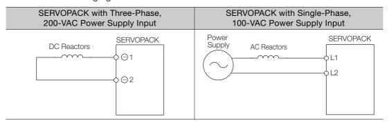
Note: 1. Connection terminals ⊖ 1 and ⊖ 2 for a DC Reactor are connected when the SERVOPACK is shipped. Remove the lead wire and connect a DC Reactor.
