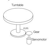
Because the turntable moves in only one direction, the upper limit to the number of rotations that can be counted by an absolute encoder will eventually be exceeded.
